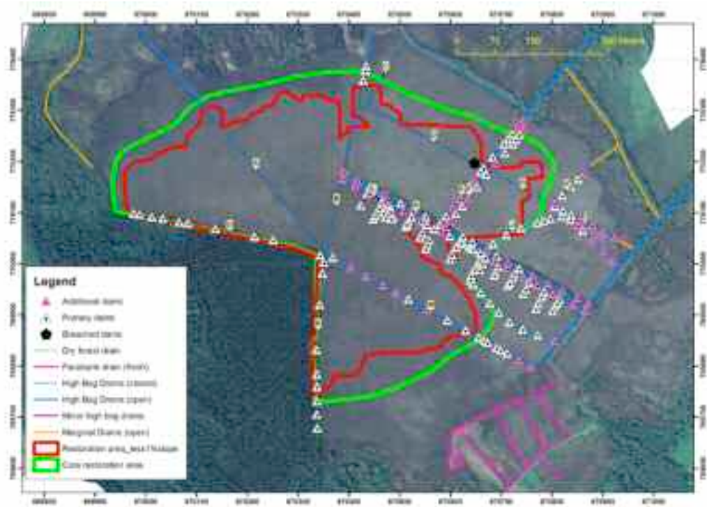
Figure 22: Restoration Plan for the hydrology and peat forming ecotopes in a central core area of Girley Bog Co. Meath 2012. The area encompasses almost all part of the high bog (11%) where the topographic gradient is less than 1%. Primary dams are located at those points where the drain elevation has dropped by 10cm. Additional dams are located in those areas where the gradient is gentler, but where at least 3 dams per 100m length of drain are required. Source: Flynn & Regan 2012.
